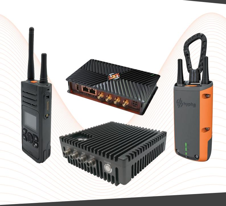
HyphaMESH solutions offer an IP transparent network, based on the COFDM waveform, that can operate independently or integrate back to a central core, wider network or the internet. This extends coverage for Wi-Fi enabled devices, sensors and cameras into challenging environments such as back country, urban or underground areas of operation.
