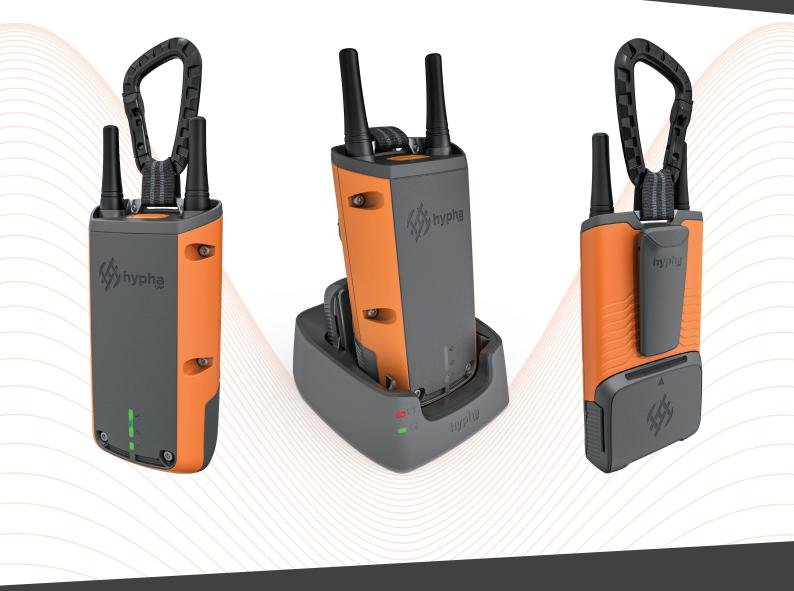
HyphaCAP is a lightweight, portable device that combines mesh and Wi-Fi technologies to enable users to connect smart devices, sensors and cameras in environments that defeat radio and cellular communications.
